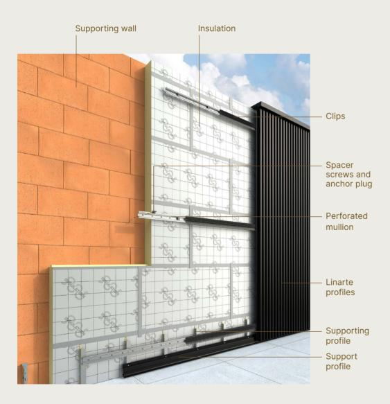
With the patented fixation system, the mullions can be directly affixed to the substructure. Compared to the traditional system using a wooden support structure, this method is more advantageous because of the lower material cost and quicker installation time. Thanks to the direct fixation, there are fewer thermal bridges, the total system depth is smaller, and you have a more sustainable solution.
